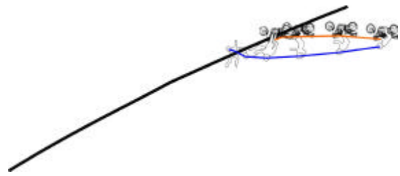
Figure 11. Trajectories determined from the overhead-view cameras of the motorcycle and the dummy before and after impacting the steel guard rail (Figure 10)
