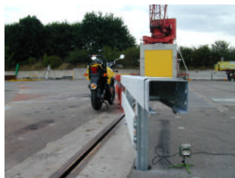
Figure 14. Modified guard rail system with respect to better protection for impacting motorcyclists
