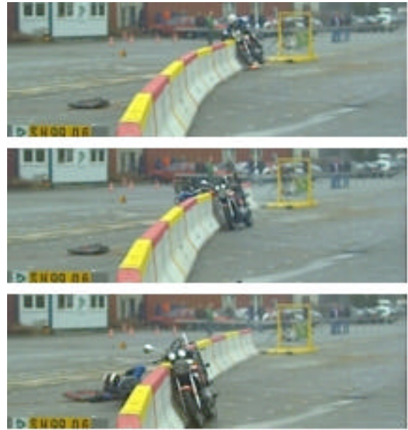
Figure 8. Full-scale crash test of a motorcycle impacting a concrete barrier protection system in an upright position prior to impact moving
