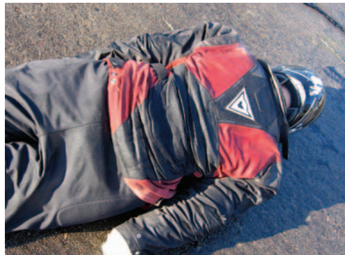
Leather or textile: 80 km/h skid tests with crash test dummies dressed in leather and textile riding gear from the same manufacturer showed no significant difference in safety performance.
