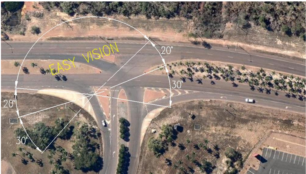
Figure 4.84: Poor visibility angles to through road
