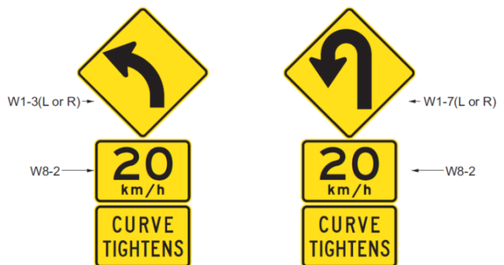
Figure 4.35: Compound curve warning signage
