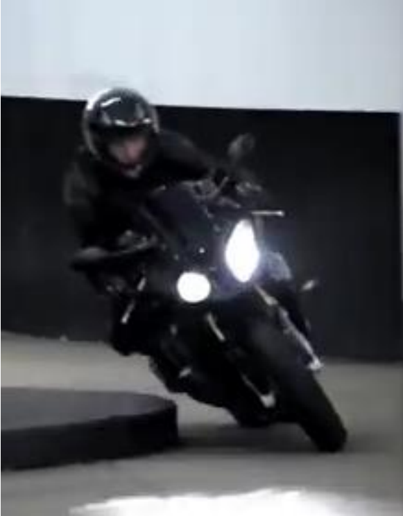
Figure 4.91: Barrier kerb on inside of motorcycle lean zone
