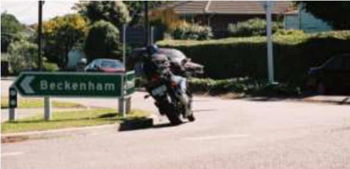
Figure 4.27: Road furniture on the inside of a turn
