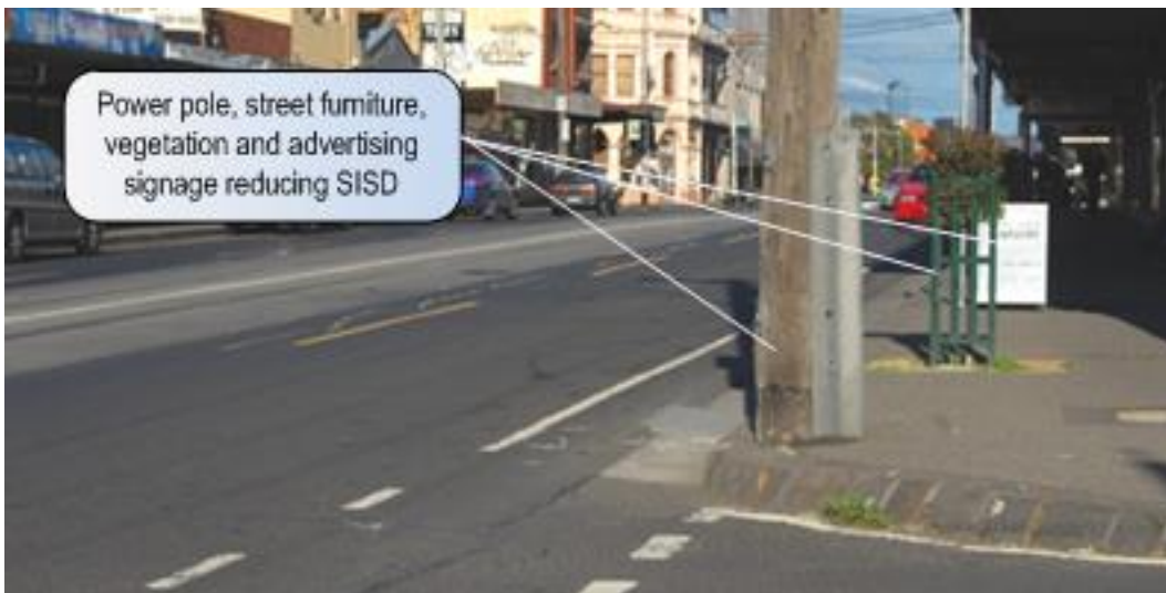
Figure 4.78: Urban – restricted safe intersection sight distance
