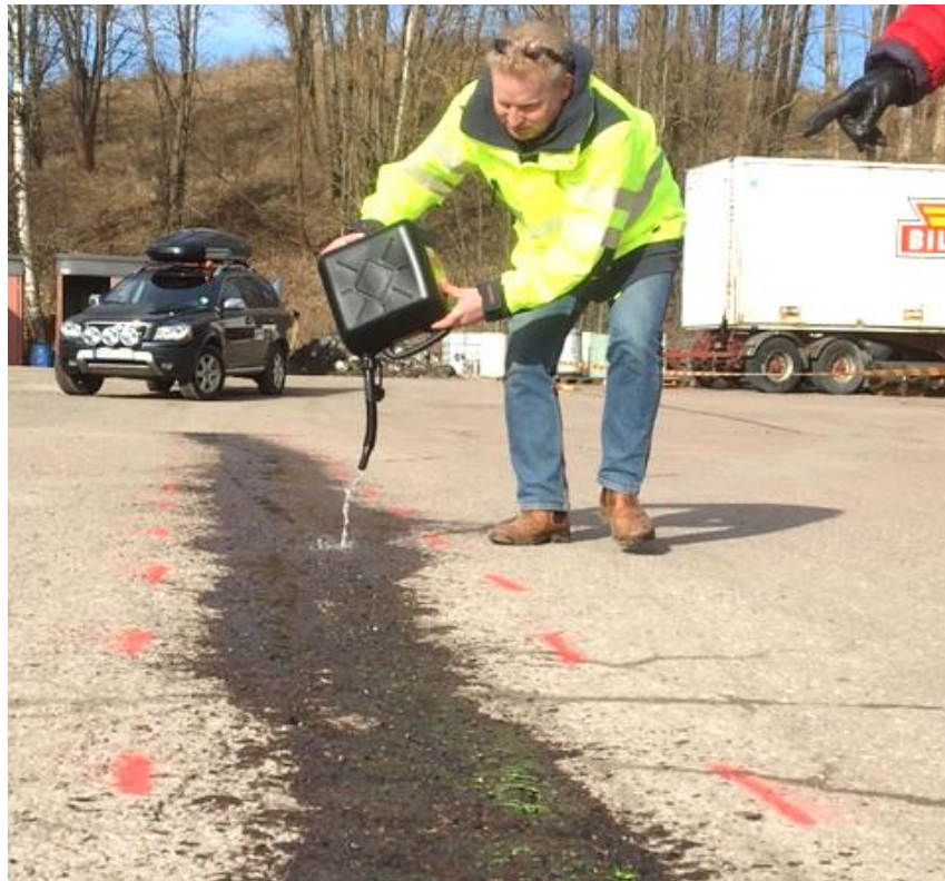
Figure 4 Spilling 10 liter diesel in the 20 m test section. Photo: P Holmlund
