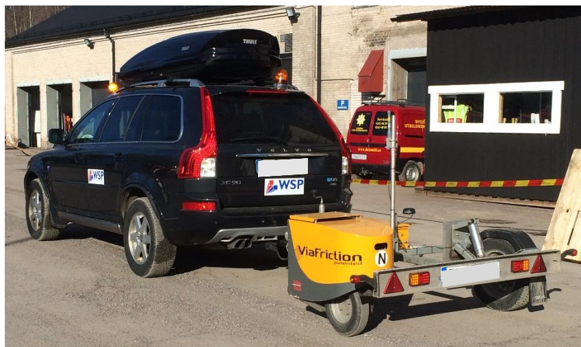
Figure 2 The ViaFriction trailer for measurement of road friction. Photo: J Granlund
