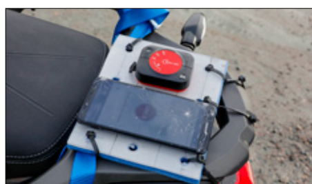
Above left: Dual Skypro XGPS160 and mobile with RaceChrono Pro mounted on one of the bikes. Above right: Measurement data is analyzed with great interest in the Racelogic VBOX Test Suite.
