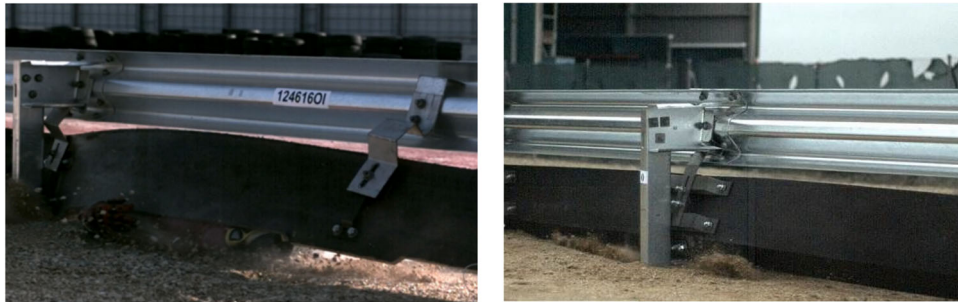
Figure 8. Arm entrapment due to the barrier raising (left), solved by the new proposed design (right).
